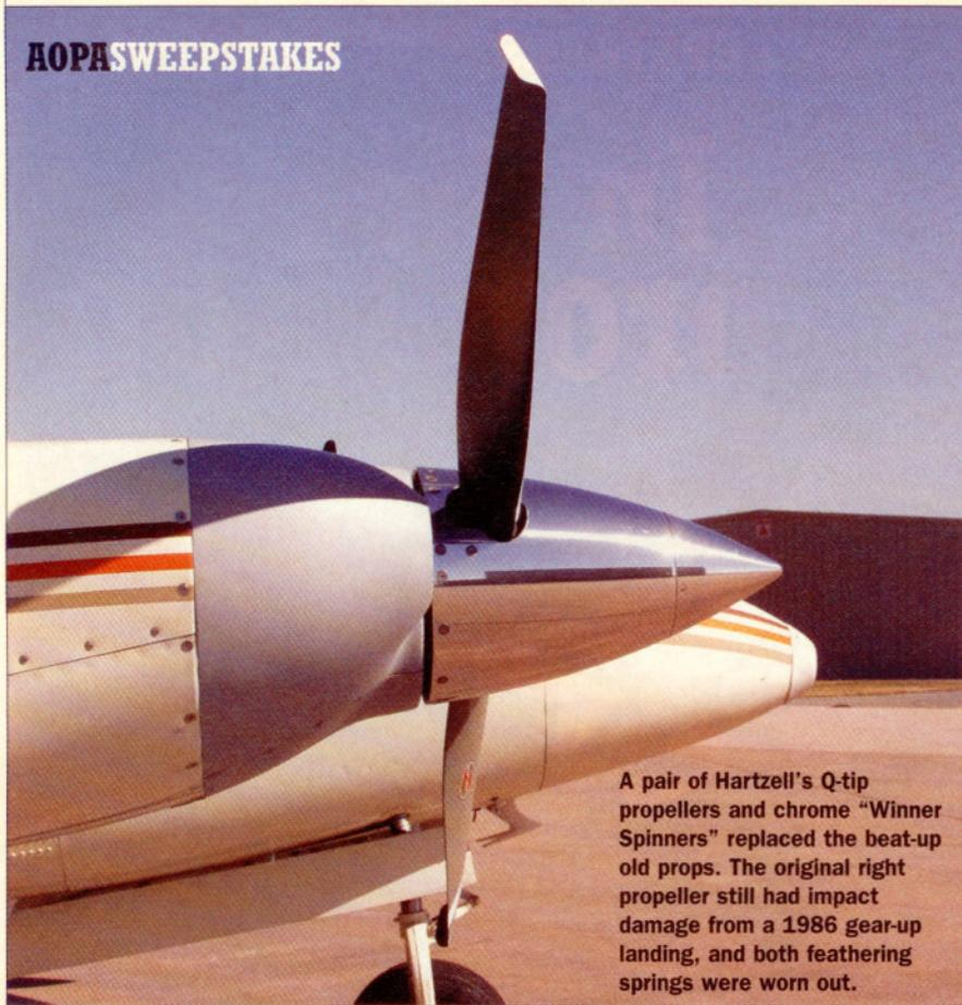
A pair of Hartzell's Q-tip propellers and chrome "Winner Spinners" replaced the beat-up old props. The original right propeller still had impact damage from a 1986 gear-up landing, and both feathering springs were worn out.
