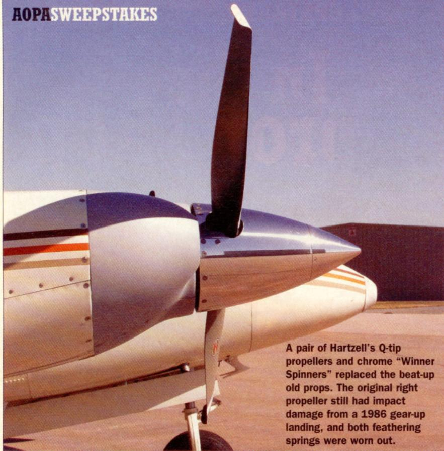
**A pair of Hartzell's Q-tip propellers and chrome "Winner Spinners" replaced the beat-up old props. The original right propeller still had impact damage from a 1986 gear-up landing, and both feathering springs were worn out.**
